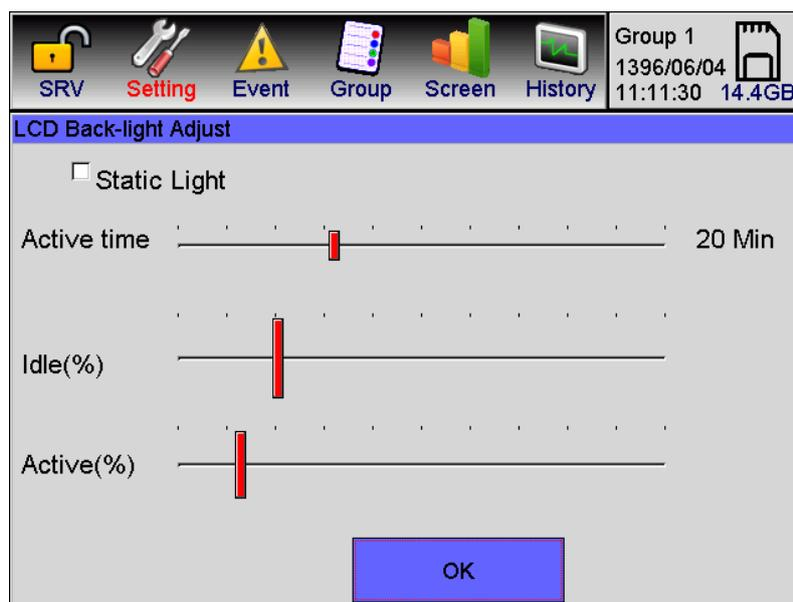
Figure 4-18: Adjust the light of the LED screen in the back light without activating Static light
