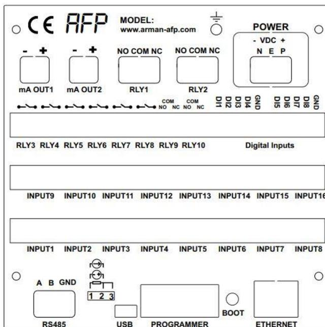
Figure 3:Connector view behind the device
