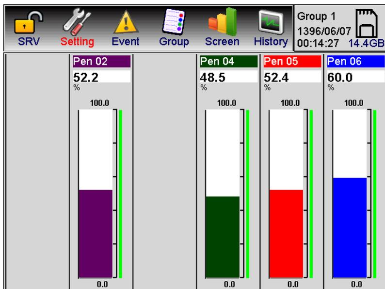
Figure 5-9: Zeroing the corresponding pen with two members and removing two pen from the page in the Vertical bar graph section.
