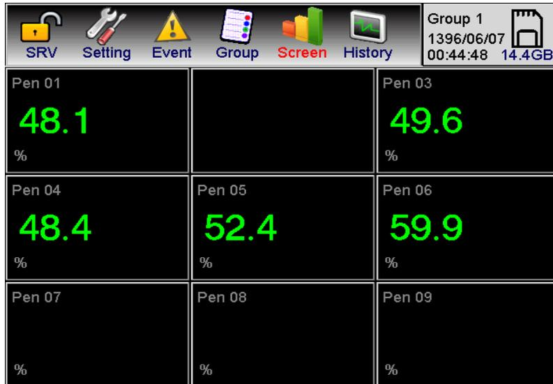
Figure 5-24: Zeroing the corresponding pen with two members and removing these two pens from the screen in the Black indicator
