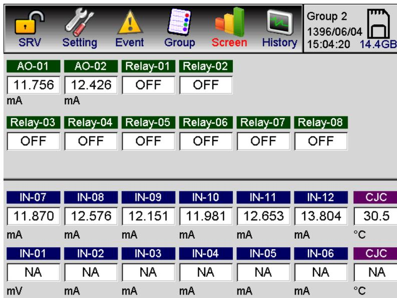
Fig. 5-25: View the instantaneous values of the electrical parameter of each input of the device in the Input overview section.
