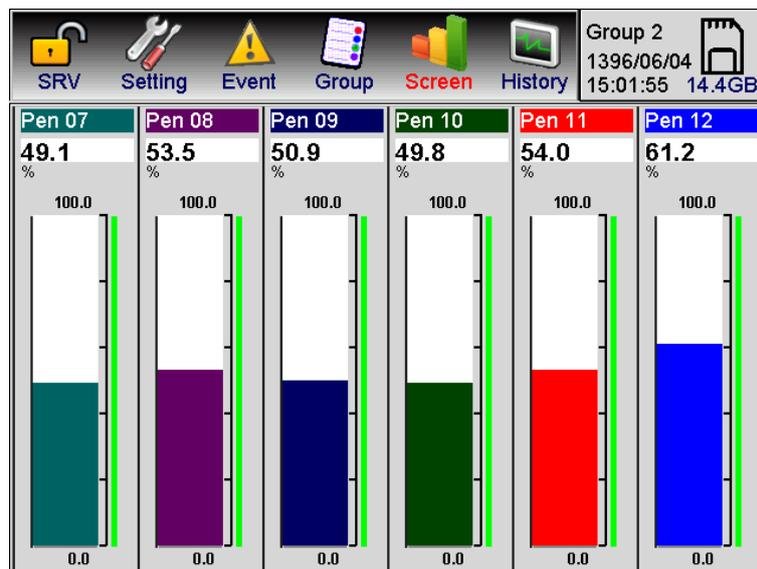
Figure 5-7: How to display the values of the pens in the Vertical bar graph
