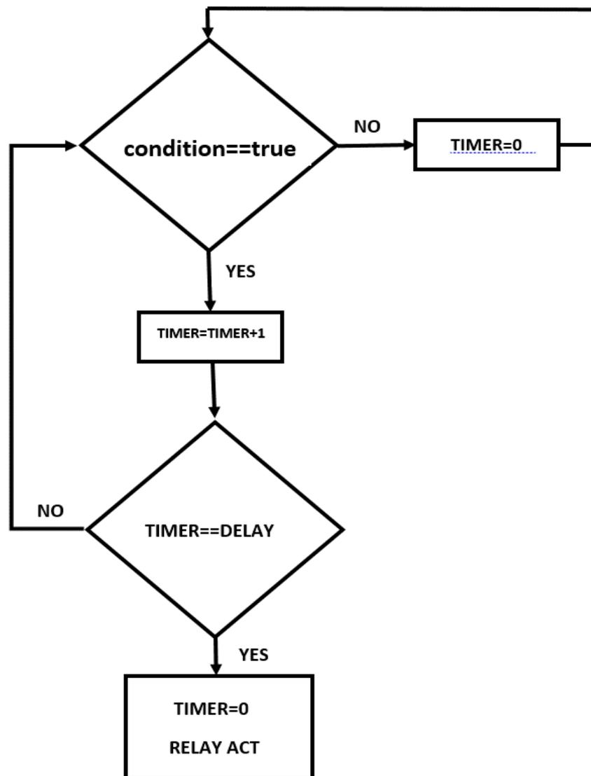
Figure 2-14: Flowchart of the Digital Output Function (Relay)
