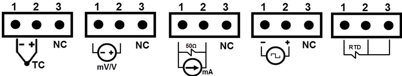
Figure 2.1: How to connect different signal types to the input connector
