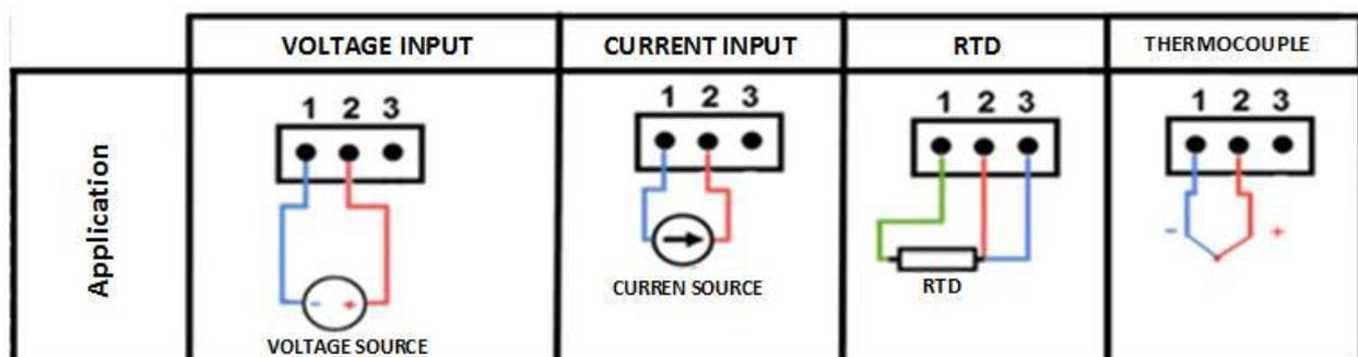
Figure A-4: How to connect signals and different sensors to inputs
