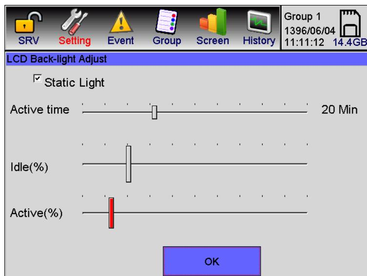
Figure 4-19: Adjust the light of the LED screen in the back light with the activation of Static light
