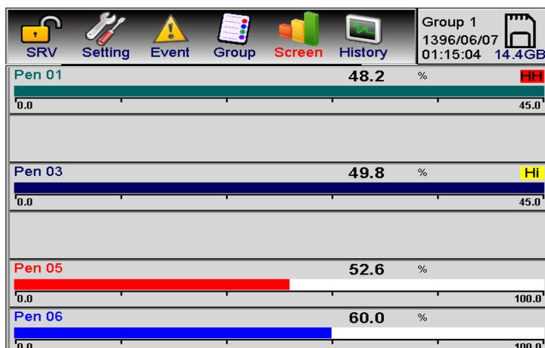
Figure 5-11: Zeroing the corresponding pen with two members and removing two pens from the Horizontal bar graph page
