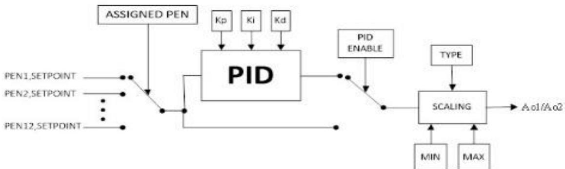
Figure 2-11: Block diagram of the analog output section
