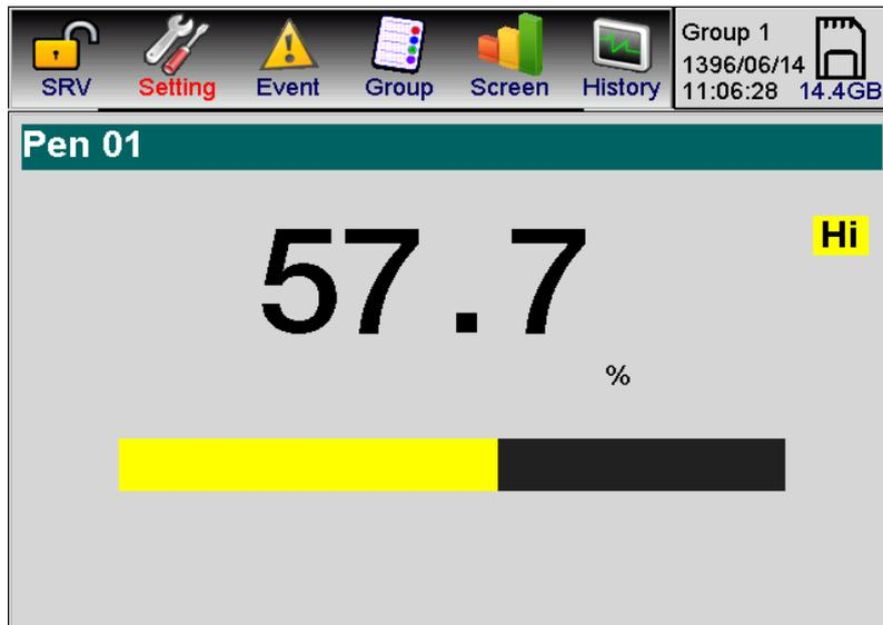
Figure 5-17: Displays the yellow color as a warning when the pen value is higher than Hi
