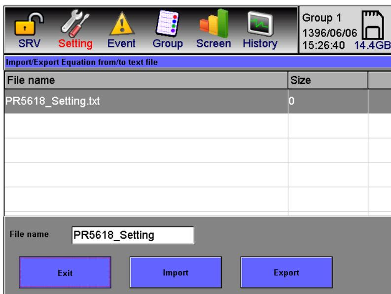
Figure 4-5: Import / Export on the CJC thermocouple Input tab
