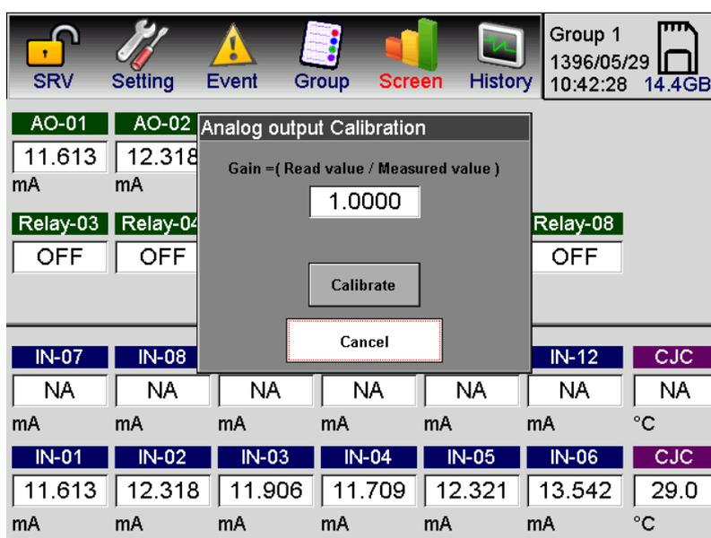
Figure C-2: Analog output calibration window
