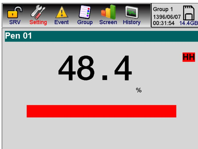
Figure G-3: Displaying alarm in Single indicator
