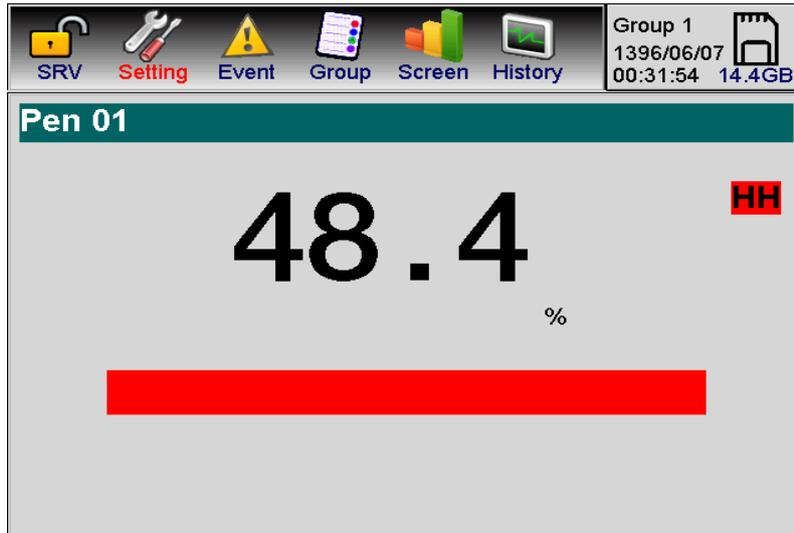
Figure 5-16: Displays the red color as an alert when the pen amount is higher than the HH value
