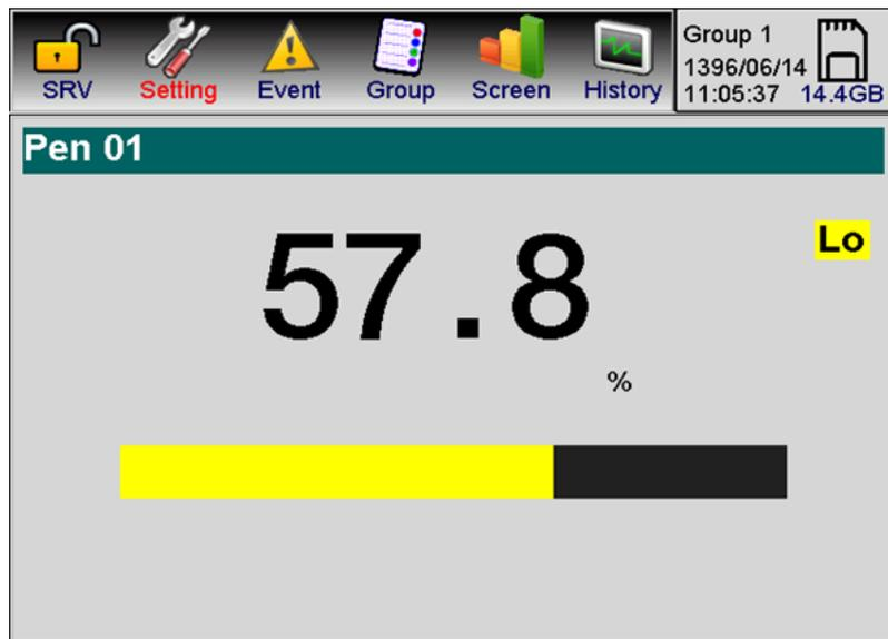
Figure 5-18: Displays the yellow color as a warning when the value of the font is less than Low
