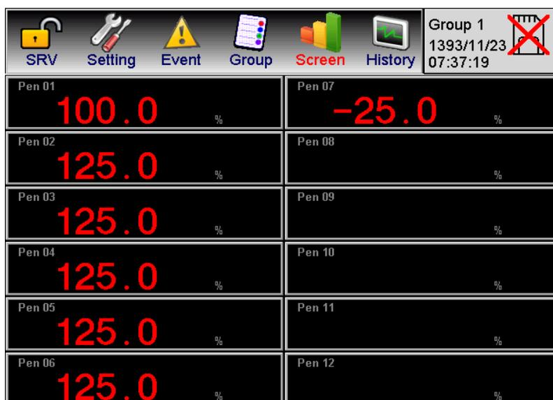
Figure 5-23: Displaying 7 of the 18 pens in the Black indicator section
