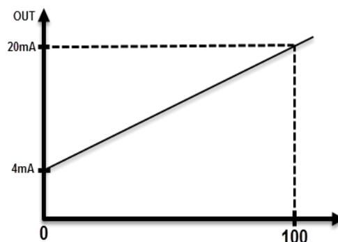
Figure 2-2: Output current range (4 to 20 milliamps) between 0 and 100
