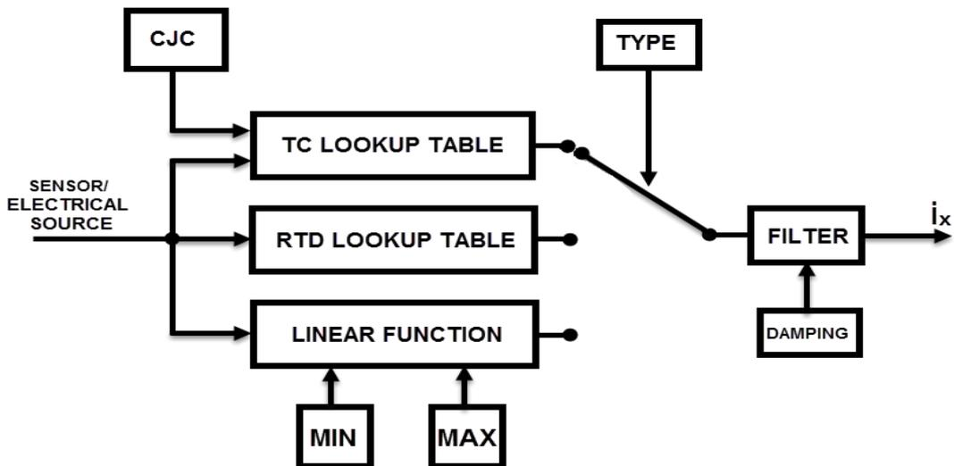
Figure 2-2: Internal block diagram of an input channel
