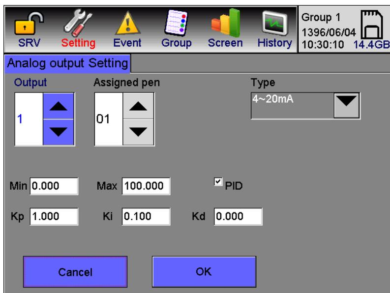
Figure 4-13: Analog output with PID controller
