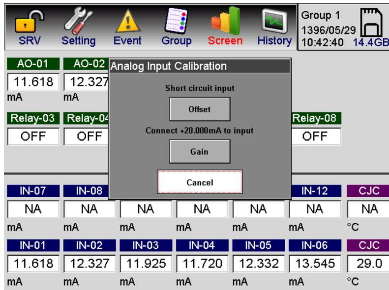
Figure B-2: Analog Input Calibration window
