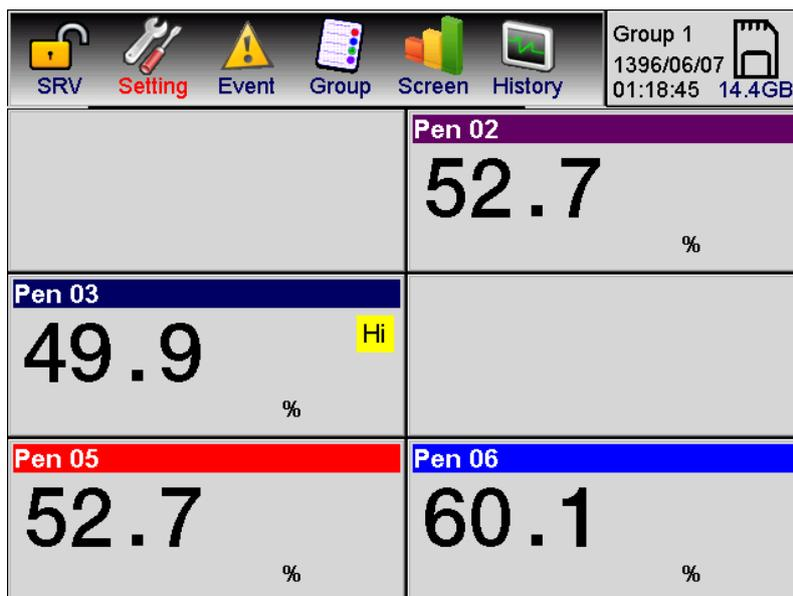
Figure 5-20: Zeroing the corresponding pen with two members and removing these two pens from the page in the Group indicator section
