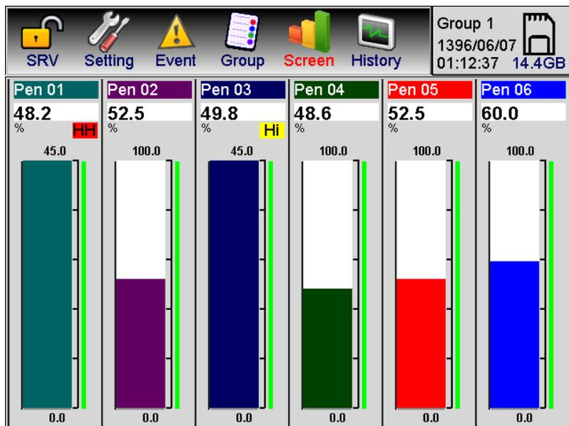
Figure 5-8: Existing alarms on a pen and the changing color according to the situation in the bar graph
