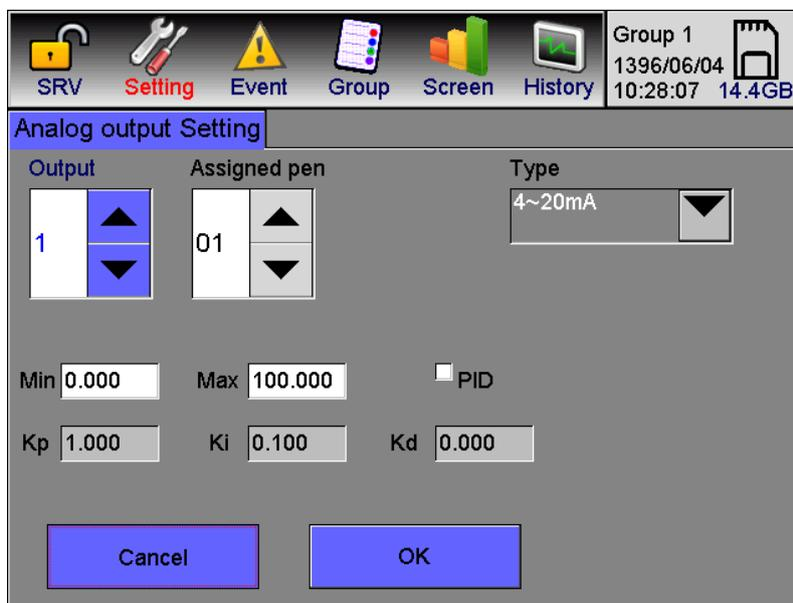
Figure 4-18: Analog output without existing PID controller
