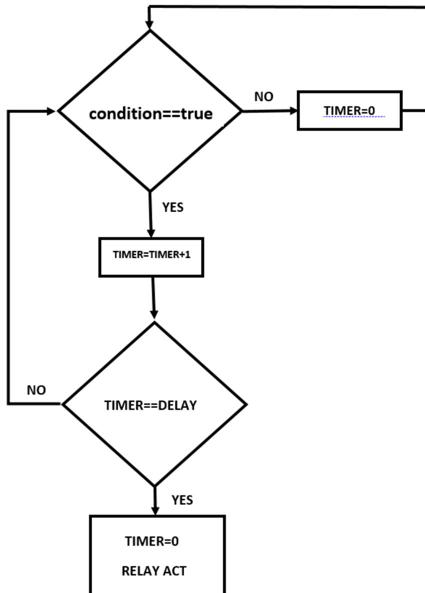
Figure C-4: How the relay outputs work
