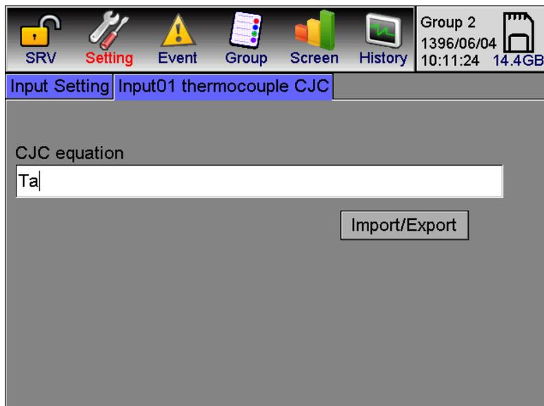
Figure 4-4: Input thermocouple CJC tab
